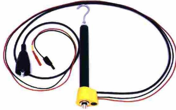
Each 15KVP is 16 inches long and 1.5 inches in diameter. They connect to high voltage lines via an open hook that is 1.3 inches in diameter. The hook is screwed into the end of the probe. It can be replaced with other custom attachments. The bottom of the 15KVP has a recessed threaded coarse 5/8" hole for mounting to a hot stick. The 15KVP is lifted into position via a hot stick. Hot sticks may be purchased from Summit Technology [order **STKS**] or may be supplied by the customer.
