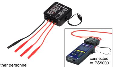
The four inputs (labeled) of the LDCm can be connected to the corresponding phases & neutral of the analyzer, from 100–480 Vrms, from 50–60 Hz without affecting the output, providing foolproof operation and maximum flexibility. The voltage leads that come included with the analyzer can be inserted into the corresponding sockets on the opposite side of the LDCm.
